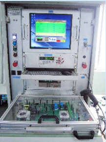
Automatic PCBA ATE test platform
